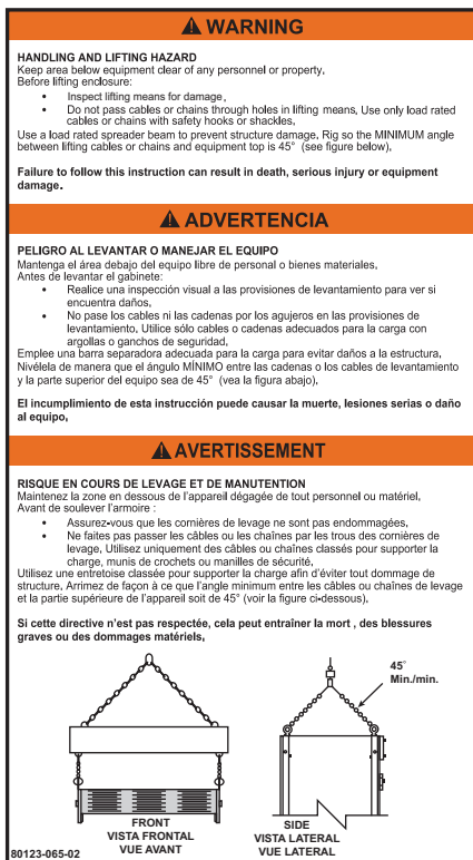
Label Applied Adjacent to Lifting Eyebolts
